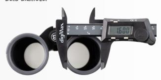
But what does the second number stand for? Quite simple: it tells you the size of the lens diameter in millimetres. This refers to the width of each lens at the front of your binoculars. The larger the diameter, the more light comes through the lens to your eye and the brighter your image will be. In these binoculars, the diameter is 42 mm. This is why the binoculars are called 8x42.
