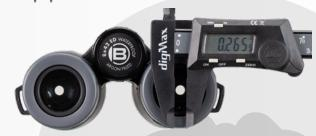
The so-called exit pupil is the bright spot you can see when you look into your binoculars from above. The larger it is, the brighter the image appears in your eye. You can calculate the exit pupil by dividing the lens diameter by the magnification: Lens diameter/magnification = 42/8 = 5.253
